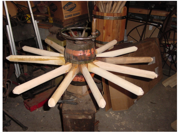
#19 Spider on wheel stand with spokes pointed
