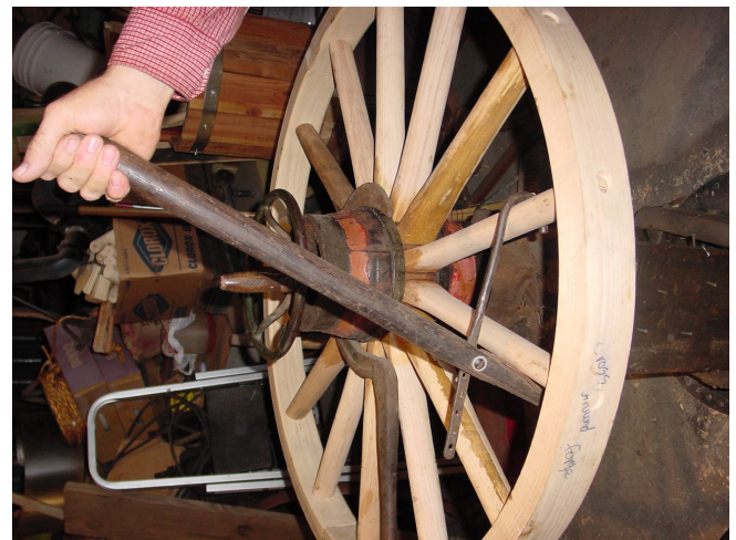
#4 Spoke puller. This is used to pull spoke into position in the felloe.
