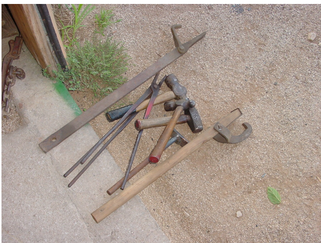
#3 Wheel Sampson. Adjustment end.
