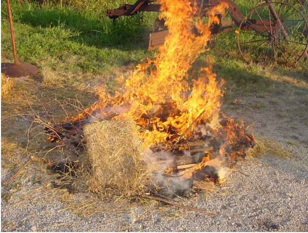
#6 Fire heating wagon tire.
