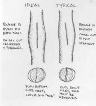
steel' to be removed with a small chisel or file.
