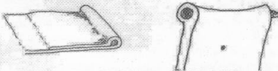
The hinge after welding. Correct bowed barrel if necessary.
