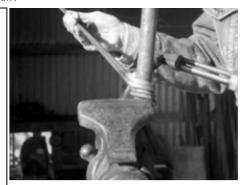
8 or Make 9 turns around the sucker rod mandrel and then let the two coils cool before you unscrew them from each other. A little WD-40 or some other light lube helps in getting them apart. If you are careful, and you made uniform coils on the mandrel, they should separate with little distortion.
