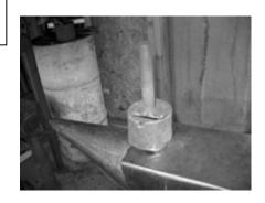
It's hard to freehand an even base around the anvil horn since the coil prevents the piece from going very far over the horn. I built little jig from scrap 2 7/8" pipe and ¾" sucker rod. Notice the little notch at the near edge of the jig.
