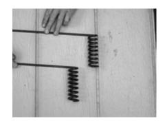
Heat the straight part of the ¼" rod, drop the coil over the sucker rod and engage the heated portion in the notch to begin forming the base. Bend the ¼" stock all the way around the pipe and you will have a nicely formed base. You should have enough rod left to form the handle of your choice.
