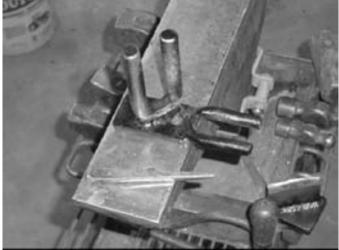
Photo O1: From these observations came the idea for the Multi-Fork you see presented here in these notes. This is simply a combination of the farriers' horizontal bending pins and traditional anvil mounted vertical bending fork. I turned the legs of the vertical fork 45 degrees to the anvil center line; it seems to be handy for me in that orientation. My cut-off hardie is also rotated the same way as this bender.
