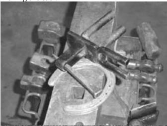
Photo O3 shows how the pin is used with a hardie stem or peg made from U-bending basic flat bar stock. For my tools that I want firmly mounted to the anvil (anvil cone for example), I have been making the hardie stems in this manner. A second benefit is that the tools are lighter than if the hardie stem was solid bar.
