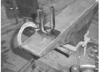
Photo O2 shows the Multi-Fork firmly pinned to the anvil. With only a light hammer tap on the tapered pin the tool is locked in the hardie hole. You can turn the anvil stand over before moving the tool.
