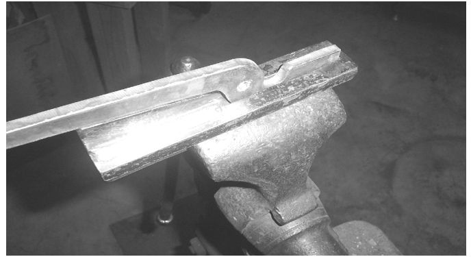
tong blank ready to shape the jaw.
