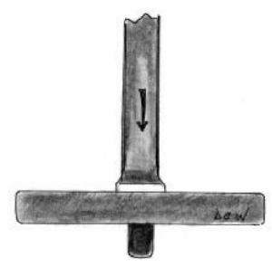
Note: The entire tenon and a bit of the shoulder must be at a bright heat to insure a tight joint.
