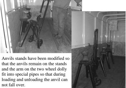
The swage block/vice stand has the same loading/unloading safety feature. And uses the same two wheel dolly. Straps (not shown) are mounted to the wall to help stabilize the anvils during travel.
