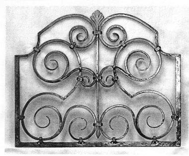
To the left is a grille designed by J C Banks. JC learned quickly the benefits of test pieces and figuring out the sequence of events. His frame has 2 corner welds, plus 2 others in the middle of those concave curves at the top left and top right of his piece. The branching scrolls with the pass-through added a challenge, made a little more interesting as the stock is 3/8 inch square.
