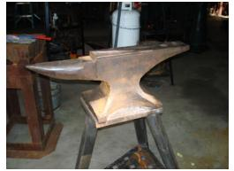
After a lot of welding, grinding, welding, grinding..... He got the anvil repaired. He then used some bleach and peroxide to even out the rust look. CAUTION do not breath the fumes of this mixture;
