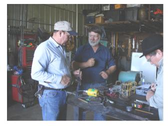
You use files, stamps and dremels to create the design. Here a dremel is being used with a small drill bit to form o's for the word LOBO. After each step in order to see who the stamp would look it was stamped into soft lead. This protected the work until it could be heat treated depending on the type of metal used.
