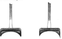
Upsetting with lighter vs. heavier hammers
