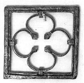
Philip Bowling from California forged a piece of wall art (right) using forge-welded branching scrolls and other techniques. His other piece (above) used 4 corner welds, a quatrefoil, with collars.
