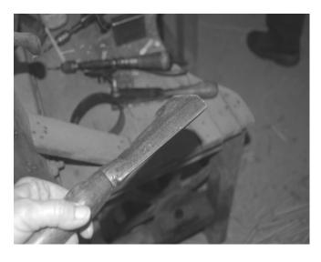
Broom making tool used to press (hammer) the wire, used to do the initial attachment of the corn to the handle, down tight onto the corn.
