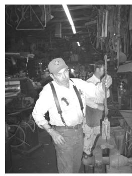
closely at the photos. John uses a piece of 2" piece of steel pipe with a handle welded to one end. This is just like the latest in commercial convection/ conduction radiation ovens. The pipe is heated in the forge to a good dull red, tapped on a heavy object at hand to shake loose any coal, coke, clinkers, or scale and then placed over a hot dog. The chief gives a good mental 10-count and the dog is cooked to perfection and ready for the bun. One heat of the pipe will cook at least two dogs. If
