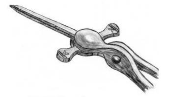
While completing the weld on the top of these nails forge a scarf from the backside as shown. First make sure the thin tops of the arms are flush on the front and then thin the shaft below the arms leaving a "bulge" on the lower half of the arms.
