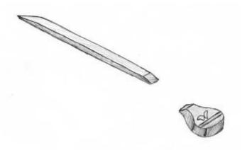
**Turn** the nail over and form the loop. Forming the loop before forge welding it to the back of the central nail gives you a means of positioning the two nails for welding and protects the tapered point while in the forge.
