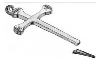
**Oh**, and remember that cast cross I set out to repair? Well I did finally get the two broken pieces back together but not without making three pieces out of two first. With persistence I finally coaxed the three pieces back together with solder and after some grinding with a Dremmel tool, filing and sanding, it looks almost like brand new:
