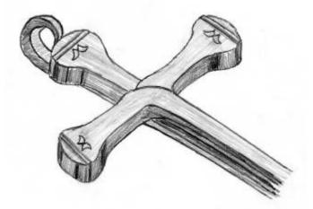
**Trim** the bottom of the cross to 2 and 3/4 inches and then upset the bottom end leaving only a slight taper (if any) in the width and thickness of the bottom of the cross with a slight swelling at the very bottom.
