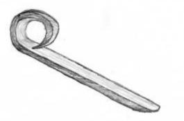
**Place** the loop tight against and behind the head of a second nail. After the cross is completed you can reposition the loop slightly so it is not tight against the head.
