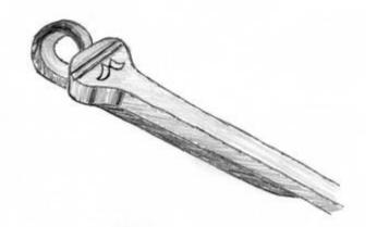
**Hold** the nails by the head and loop. I used a pair of Round bit Farrier's Fire Tongs that have domed bits that will accommodate the head and loop while holding the two nails firmly just below the head and used a tong clip to hold them secure.
