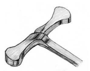
Align the arms on the central nail and forge a slight indentation to accept the bulge on the arms.
