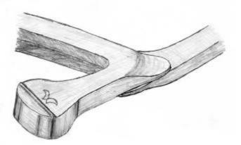
**Place** the nails in tongs and weld the points first following the same procedures as for the central nail and loop.
