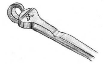
With the arms and central shaft positioned repeat the forge welding process one last time to join the two parts of the cross together. Again after welding, thin the central shaft of the cross below the arms while maintaining the proper width and cleaning up the sides.
