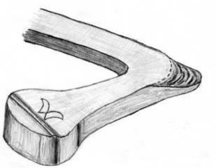
**Forge** the scarf on one nail face up and the other face down, so that when the two nails are placed together (both face up with their shanks on top of each other) their scarfs will over lap as shown here.
