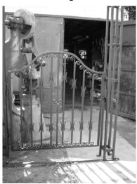
riveted on. The gate hangs between two post made from four pieces of 1 inch tubing. The space between each piece of tubing will be filled with a section of flat sheet steel with cutouts spaces along the length. It is painted black. Should be very sharp looking when
