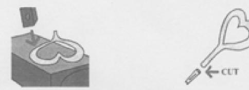
Now I start beveling the top of the curves to spread the heart and give it some character and definition. Also, takes out the twist marks. I do this by holding my hammer at an angle and hitting straight down. Start from the center of the bar and working outward at the edge of the anvil face.
