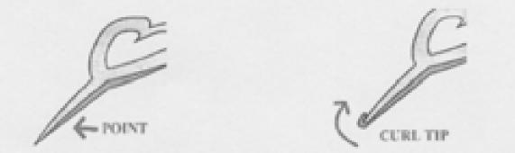
Now we are going to draw out the piece which serves as the point that forms the hook. When you are working a weld, keep it at or near a welding heat to keep from beating your weld apart. With the the tapered side of the heart up, curl the very tip of the hood point down.
