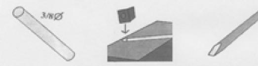
For this piece I am using 3/8" Round. The same technique can be used on whatever size heart you want to make. This is going to be a simple hoek, I also use them for a wall sconce out of larger stock, Candle Holders, a key chain fob out of smaller stock. We scarf the end of the bar and prepare it for welding.
