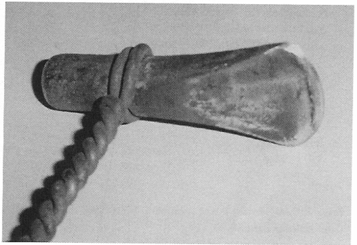
Close up of treadle hammer Hot Cut.
