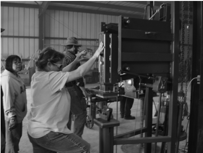
JC's treadle hammer makes short work of the offset. Aniela Hadick is trying the V-Jaw making Jig that Bill Davis fabricated.
