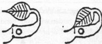
Using a bending fork, bend the leaf through 180 degrees, then bend the leaf forward so it lies over the top of the smooth curve but does not block the counter-sink depression. Mirror-image the other leaf.
