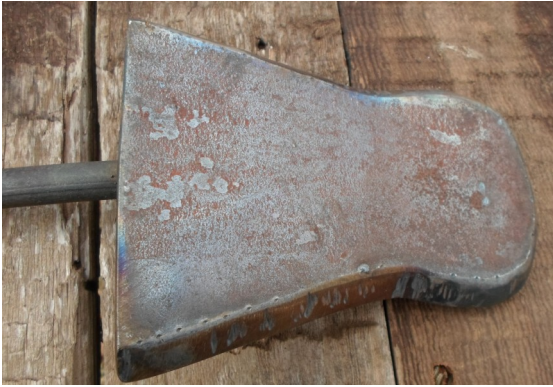
Top form for shovel. Made from 3/8" flat with a bevel of approximately 45 degrees.
