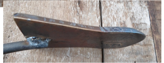
Top form for shovel. Made from 3/8" flat with a bevel of approximately 45 degrees.
