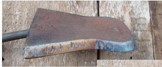
Top form for shovel. Made from 3/8" flat with a bevel of approximately 45 degrees.
