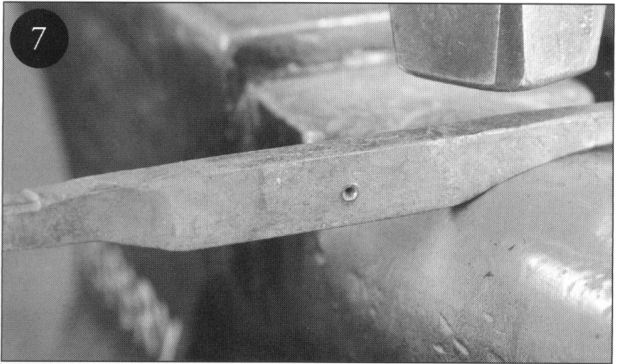
The center punch mark in the center of the bar helps to fix the degree of taper
