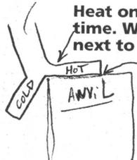
Use your anvil face as a measuring device when tapering to ensure even lengths of each tine.
