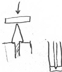
In the first heat, make a groove. Then cut twice, one side, 1st groove. Other side, 2nd groove in line with the first. Then split.
