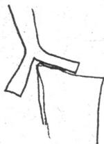
Heat only one end at a time. Work the section next to the V first.
