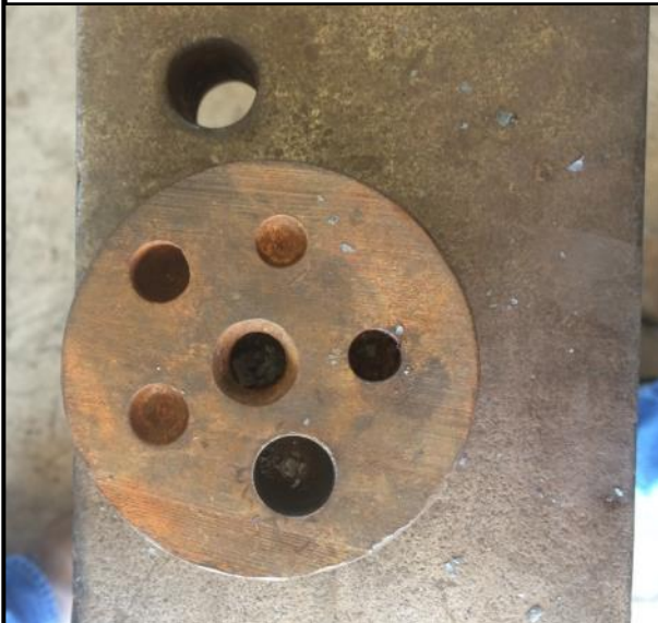
The base guide with partially drilled holes...
