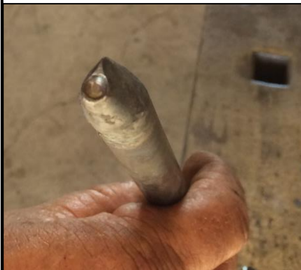
Finished eye punch ground to a teardrop shape
