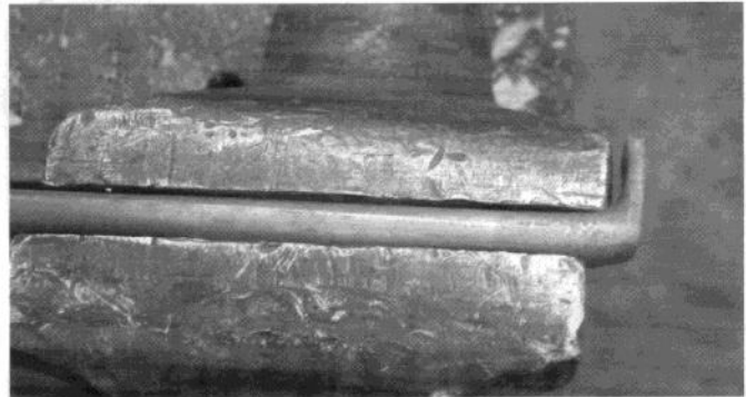
Forged shoulders on each end of the 3/8" rod.
