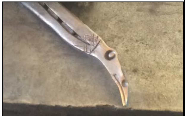
An eagle head horseshoe hoof pick made using a plain round eye punch.
