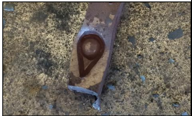
A test impression of the teardrop shaped punch on scrap stock.
