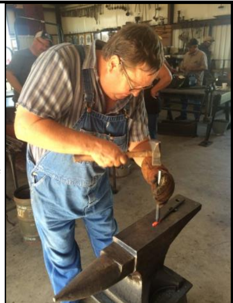
Mandell making a test impression with a newly ground punch.
