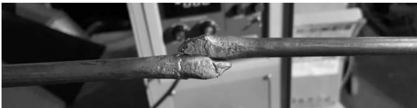
\frac{3}{8} " stock scarfed, heated and "stuck" - held only at the left end
