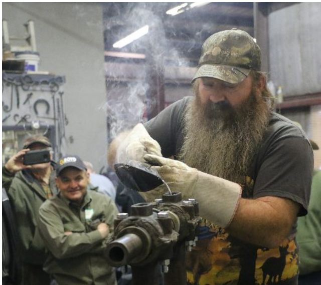
Pouring babbitt for a new upper bearing
