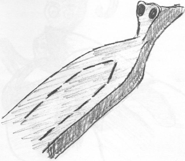
**Bend** the tongue forward and the sides of the mouth back to allow access to clean up the edges of the tongue with a file before forging to shape.
