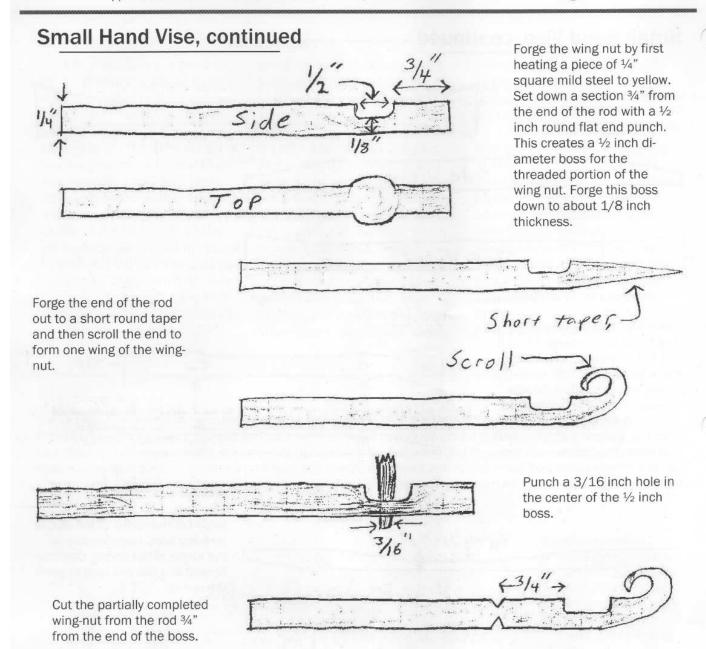
Draw the other wing out to a short round taper and scroll it just like the first wing. Drill the previously punched hole out to 7/32" and thread to  $\frac{1}{4}$ -20.
