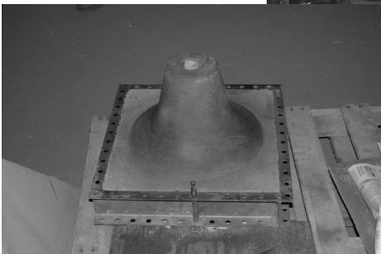
These are the two halves of the mold for the bell.
