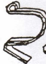
Fold the rear of the hook through a right angle (take care not to crush the hook)
