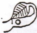
Using a bending fork, bend the leaf through 180 degrees, then bend the leaf forward so it lies over the top of the smooth curve but does not block the counter-sink depression. Mirror-image the other leaf.
