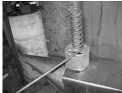
This shows the finished holder with a simple loop handle. You could add a drip pan for an extra touch. The candle in this pic isn't trimmed yet. I buy the 8" "Federal" type candles and trim about 2" off the bottom. The "Federal" candles aren't tapered and fit the 7/8" coil of the holder nicely. You can also use the 3/4" "Emergency" candles if you can find them.
