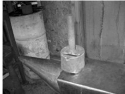
It's hard to freehand an even base around the anvil horn since the coil prevents the piece from going very far over the horn. I built little jig from scrap 2  $\frac{7}{8}$ " pipe and  $\frac{3}{4}$ " sucker rod. Notice the little notch at the near edge of the jig.
