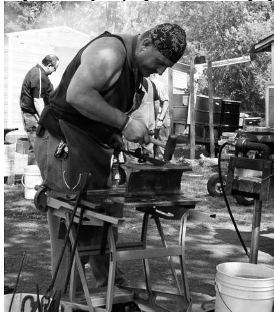
You can see from this setup that you don't have to have a fancy anvil to do blacksmithing. This is a piece of I-beam held secure in a shop mate. And his hammer is not a fancy hammer either. Just a shop hammer of an adequate weight.
