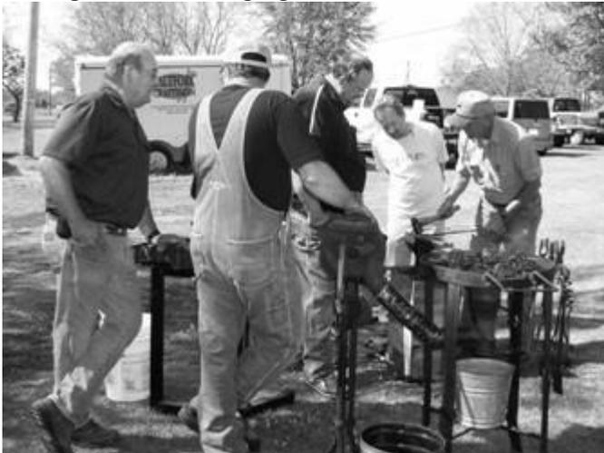
Larry Mills working on a tool using the power hammer with a swedging tool set over the lower die of the hammer?
