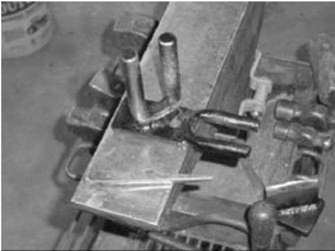
**Photo 01:** From these observations came the idea for the Multi-Fork you see presented here in these notes. This is simply a combination of the farriers' horizontal bending pins and traditional anvil mounted vertical bending fork. I turned the legs of the vertical fork 45 degrees to the anvil center line; it seems to be handy for me in that orientation. My cut-off hardie is also rotated the same way as this bender.
