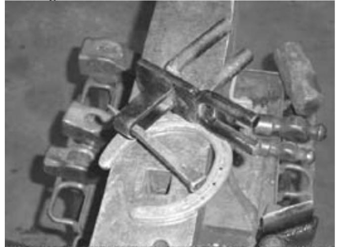
**Photo 03** shows how the pin is used with a hardie stem or peg made from U-bending basic flat bar stock. For my tools that I want firmly mounted to the anvil (anvil cone for example), I have been making the hardie stems in this manner. A second benefit is that the tools are lighter than if the hardie stem was solid bar.
