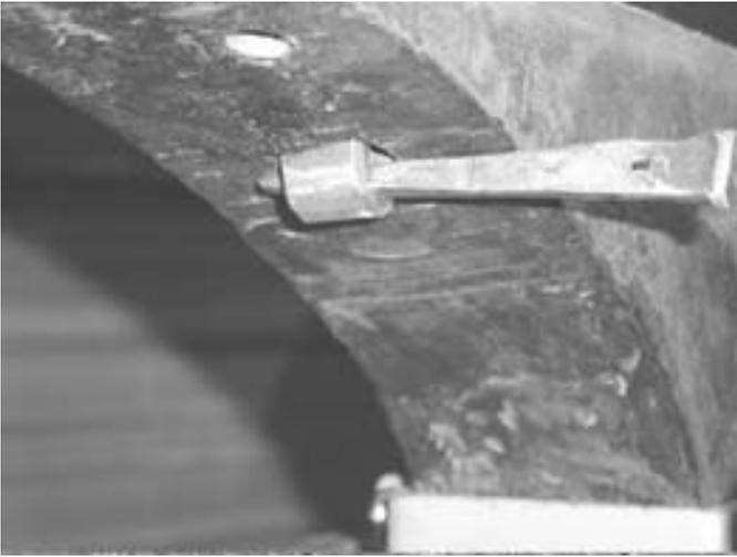
Photo 04 shows the end of the U-shaped hardie stem and the tapered pin as seen from the underneath side of the anvil heel. I really like this old Trenton anvil, but the factory did not do any finishing work to the under sides of the heel or the horn.
