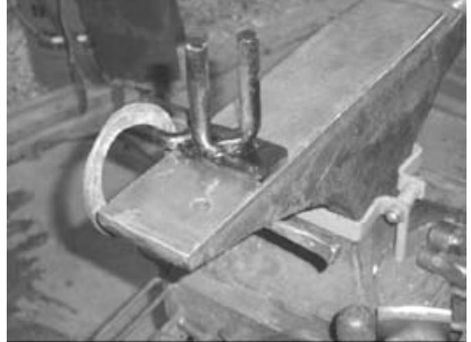
**Photo 02** shows the Multi-Fork firmly pinned to the anvil. With only a light hammer tap on the tapered pin the tool is locked in the hardie hole. You can turn the anvil stand over before moving the tool.
