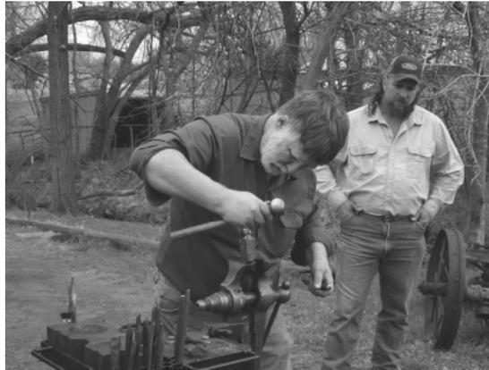
forge the Bobcat head out of Aluminum Bronze. The Bronze is harder to forge because of the limited forging temp. it was even harder to see the temp forging outside.
