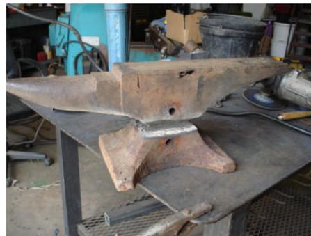
He marked how far to grind back for the bevel needed to get a good weld job.
