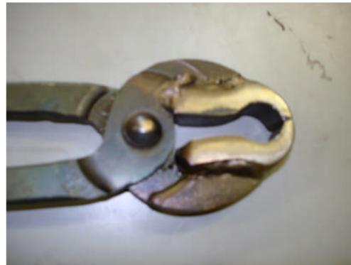
Picture on left shows the forming of the groove using the air hammer. Picture on the right shows the modification of the poz tongs.
