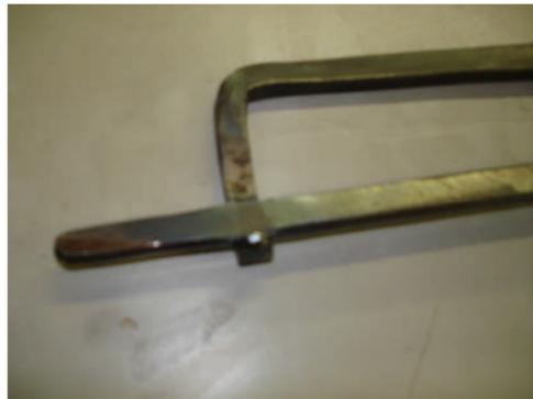
A second modification to the tong was the forming of a locking clip on one rein that allowed you to lock the tongs on to a tool.
