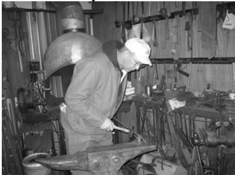
Jim Carothers needed a nail header so Ron cut a blank out of a grader blade and they went to work. After a few heats and some sledghammer work Jim had a nice functional nail header with only a little clean up work remaining.
