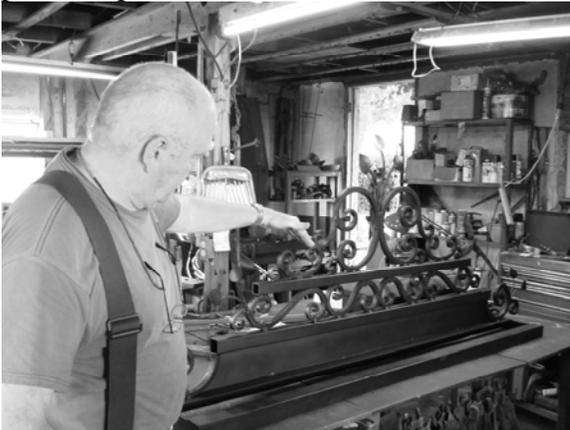
This is the top of the arch. It will have the date and other lettering that is cut from polished brass and riveted on. The gate hangs between two post made from four pieces of 1 inch tubing. The space between each piece of tubing will be filled with a section of flat sheet steel with cutouts spaces along the length.
