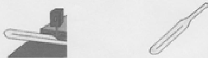
I forge weld these, but you can tack it with a mig, flux it, bring it up to a welding heat, and hammer the weld out any few know the difference. When welding this you don't want to thin the weld down too much. Center it back up like shown here.
