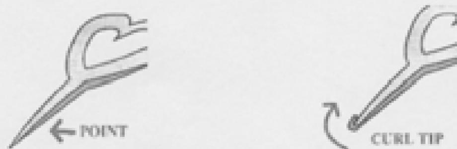
Now we are going to draw out the piece which serves as the point that forms the hook. When you are working a weld, keep it at or near a welding heat to keep from beating your weld apart. With the the tapered side of the heart up, curl the very tip of the hood point down.
