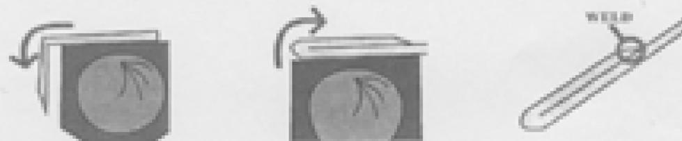
Fold the piece over the side of the anvil 90 deg. and back over itself and weld it. This fold is about 5" because that is the width of my anvil face.
