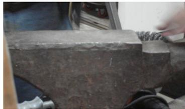
welding on the more damaged anvil. Once they were built up enough, they were ground down to the desired finish.
