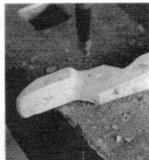
Back-punch on the face of the anvil with the jaw protected from damage
