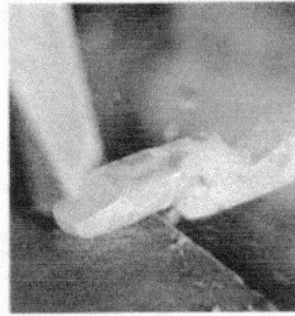
The end is drawn to a slight taper
