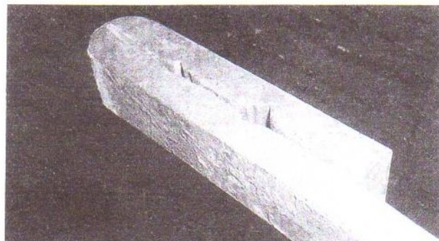
Forging the vise pads
