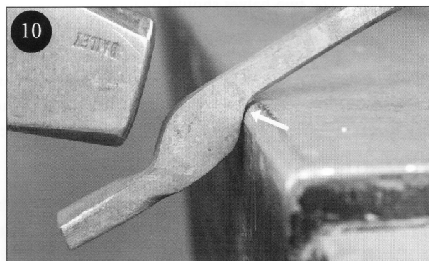
Round up the boss using a heavily relieved edge of the anvil face. A sharp edge may cause cracking later
