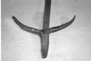
Shop Tip -- Cleaning ScrollsJim Carothers09-23-2014Cleaning fire scale out of a blacksmith made scroll can be difficult.Paint or other finishesapplied over scale often flake off later making your work look bad or making more work foryou.
