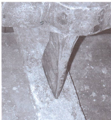
FIG 1. - DRIVE THE SLOT-PUNCH UNTIL YOU CAN FEEL THE ANVIL RESISTANCE AND STOP, COOLING THE PUNCH EVERY COUPLE OF HITS
