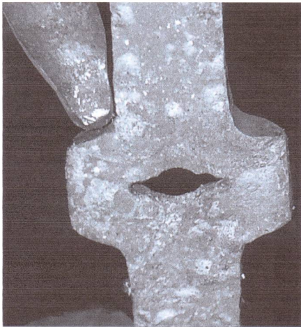
FIG 9. - ADDITIONALLY, THE OUTSIDE CORNERS CAN BE CLEANED UP AT THIS TIME USING FULLERS OR OTHER SUITABLE TOOLING
