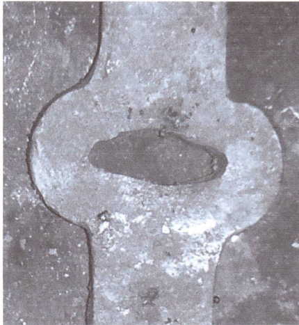
FIG 7. - RESUME UPSETTING UNTIL THE HOLE BECOMES AN OVAL
