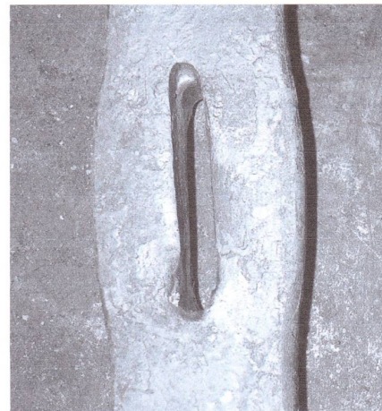
FIG 3. - MOVE TO THE HARDY-HOLE OR BOLSTER AND CLEAR THE SLUG FROM THE SLOT
