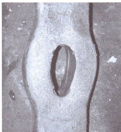
FIG 4. - UPSET THE SIDES OF THE SLOT AND CAUSE THE LONG NARROW SLOT TO TAKE ON AN OVAL AS THE SIDES MOVE OUTWARD AND THE ENDS OF THE ORIGINAL SLOT BECOME CLOSER
