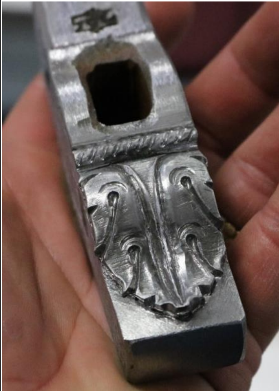
The acanthus leaf decorated hammer head with rope detail forged by Tom Latane'
