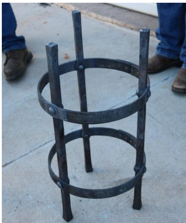
The finished riveted table project. Gerald said that the tables he sells are made in the same way but are larger in diameter and may use proportionally larger stock
