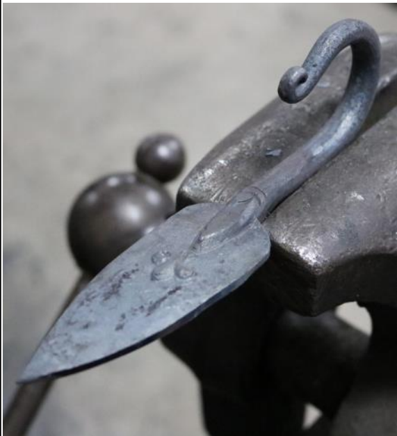
Example of a wall hook made using the fleur de lis bottom swage to accent the transition area
