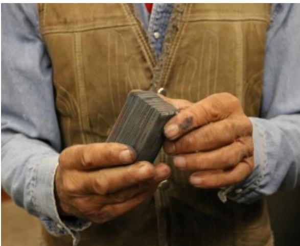
Fig. 9: The newly welded billet. Note the uneven edges which must be ground before forging.
