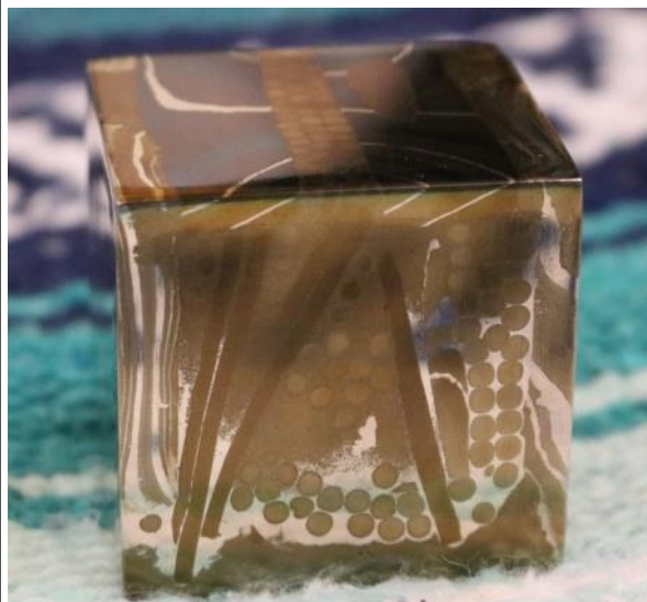
Fig. 12: A square billet made with scraps of old billet, metal powder, and steel shot.
