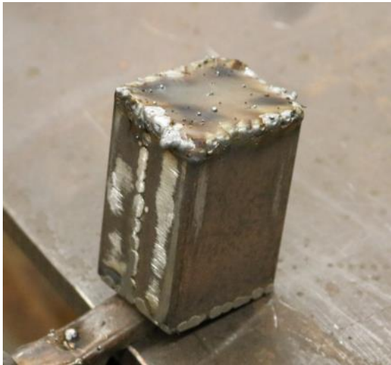
Fig. 5: The completed box with the ends welded and ready to go to the forge.
