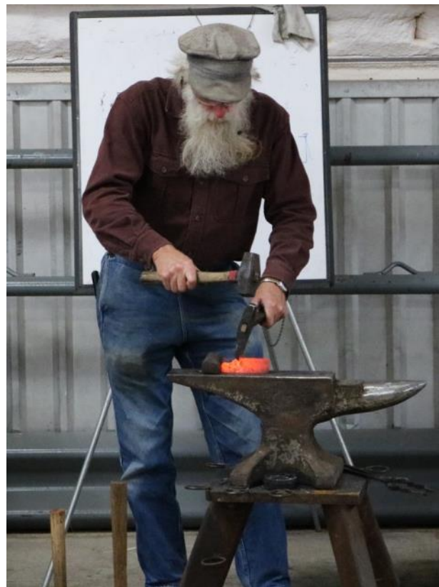
Tom Latane' forging a hammer head in preparation for decorating the head with an acanthus leaf engraving
