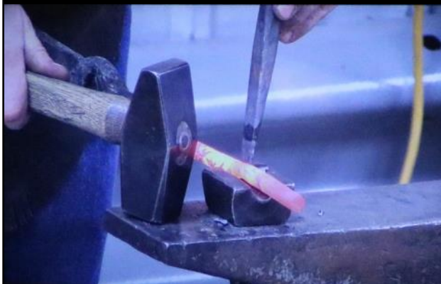
Gerald punching round stock with a round bottom swage to protect the bar
