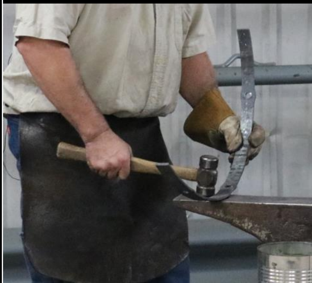
Bending the circles for the table project by hammering over the hardy hole with blows at short equal intervals
