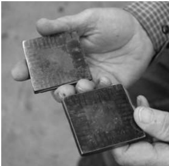
Fig. 15: Cut off box ends showing an example of a different pattern by packing layers perpendicular to each other.
