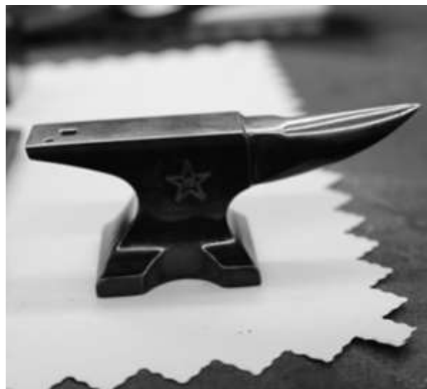
Fig. 14: This pattern welded billet anvil with tool steel face is about 1 1/2" tall.
