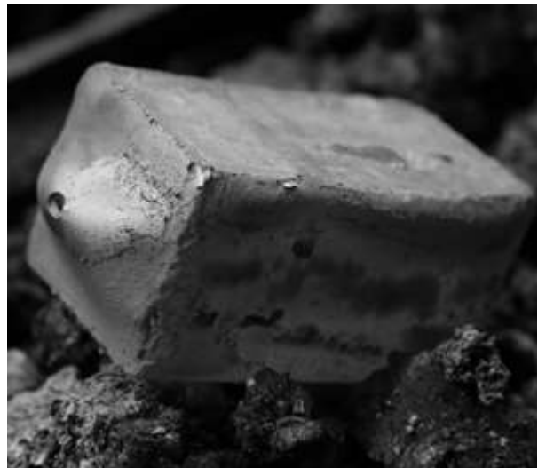
Fig. 7: The forge welded box cooling slowly in a cold coal forge. Note the small hole in the box.
