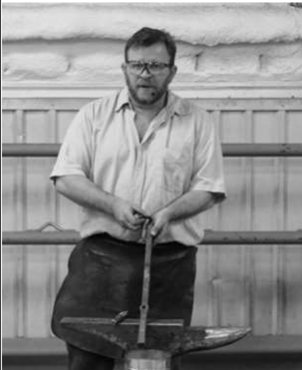
Punching and drifting upset square bar for the legs of a riveted table project
