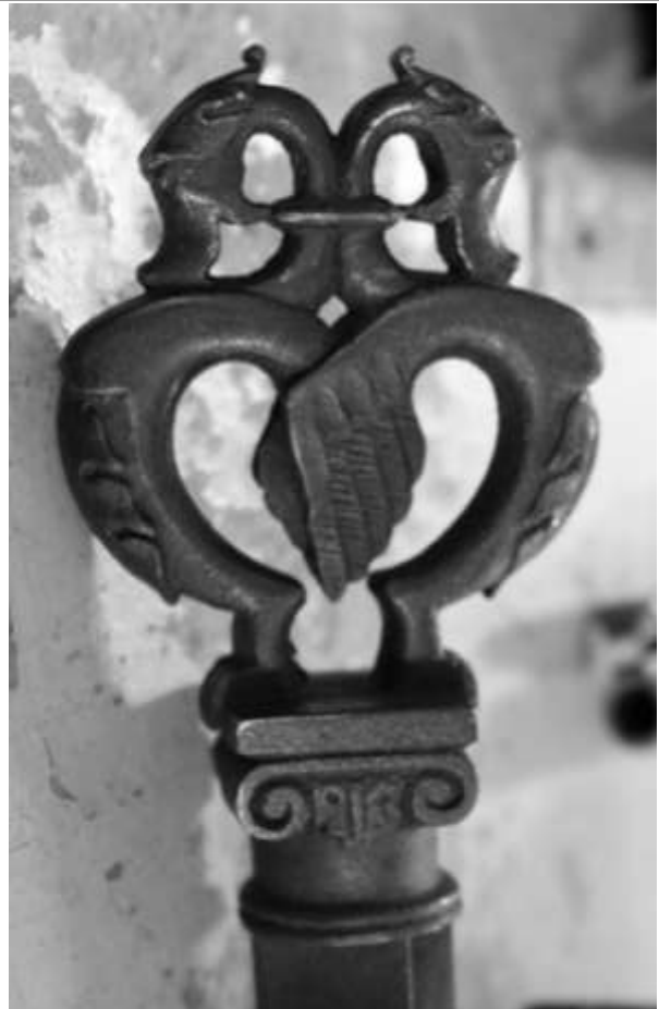
The handle end of a gothic type key made by Tom Latane'. The dragons were made by drilling, filing and chasing with chisels.
