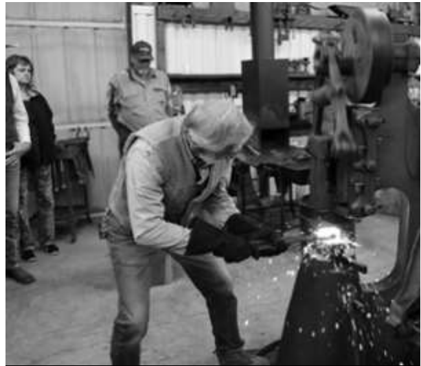
Fig. 6: Gerald forge welding the billet. Three quick hits with the 100 Lb Little Giant.
