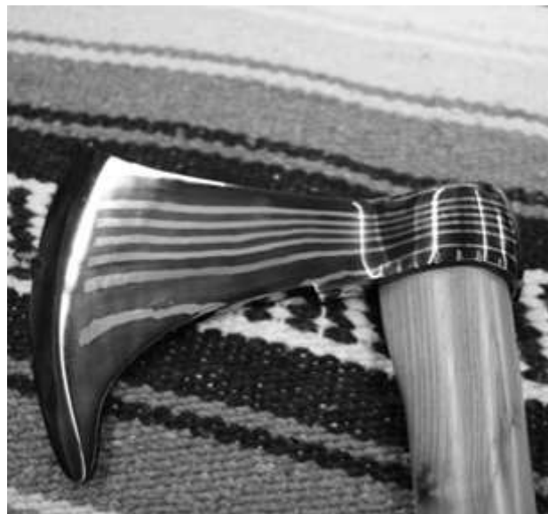
Fig. 10: A Tomahawk by Gerald. This one has 1084 welded in for the cutting edge.
