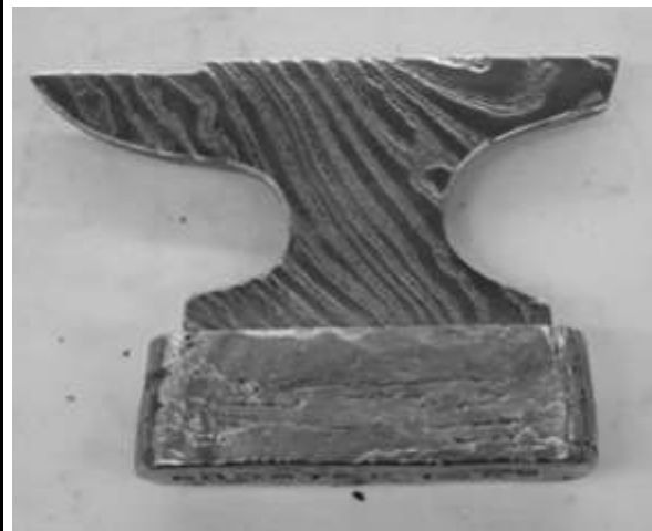
Fig. 1: Gerald's first attempt at pattern welding from 1968. Wrought Iron and O1 steel.
