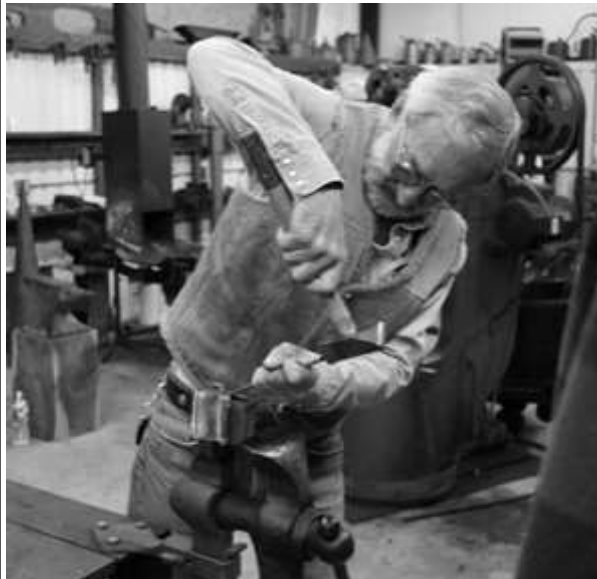
Fig. 8: Chiseling the box off to reveal the newly welded billet.
