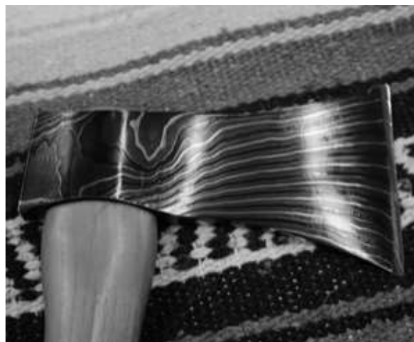
Fig. 2: A single bit axe by Gerald. Note the wide bands and dramatic contrast of layer colors.
