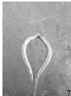
7 Continue spreading on the anvil horn. Spread the outer end most.
