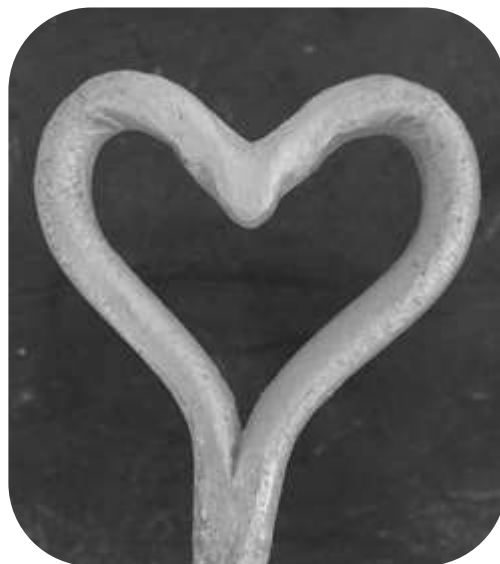
6 Begin spreading loop with a chisel. Avoid stressing the weld. Gripping weld with tongs while spreading can help if needed.
