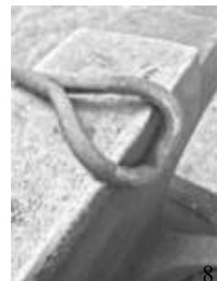
8 Bend outer 1/3 of loop on rounded edge of anvil then turn over and roll point in on anvil face until you have a flat heart shape. Fine tune curves on the horn as required.
