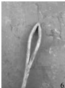
6 Begin spreading loop with a chisel. Avoid stressing the weld. Gripping weld with tongs while spreading can help if needed.
