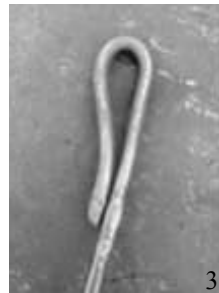
3 Bend scarf flat against upset area, heat, clean and flux.
