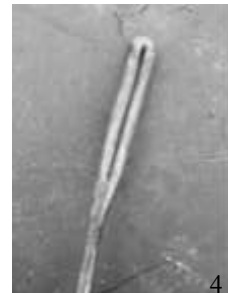
4 Forge weld joint and then flatten out the remaining loop.
