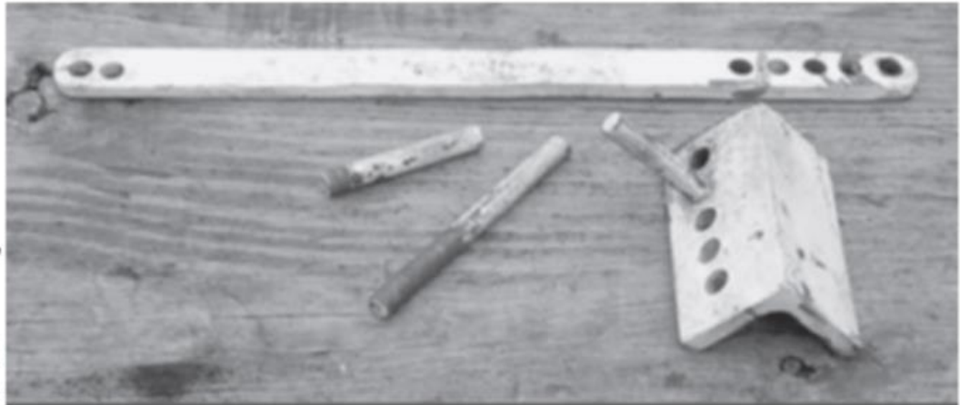
Bender parts, handle, base, three pins
