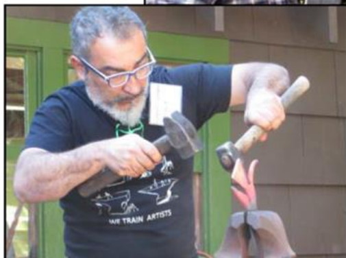
Cut lines drawn, do not make the mid part too thin, it becomes the stem.
