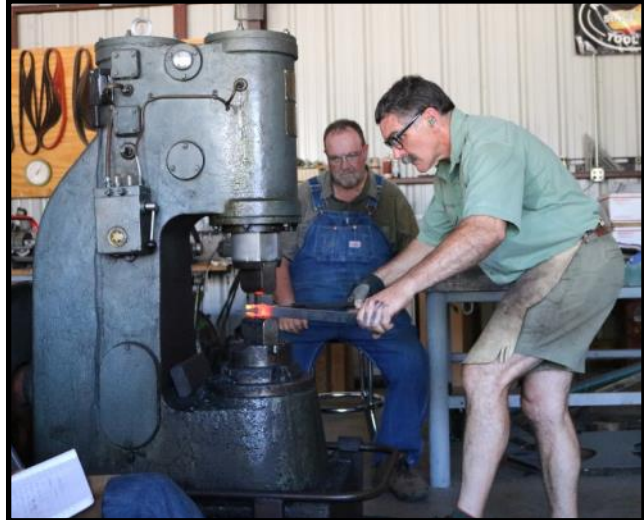
Mark drawing out the cheeks of the leafing hammer
