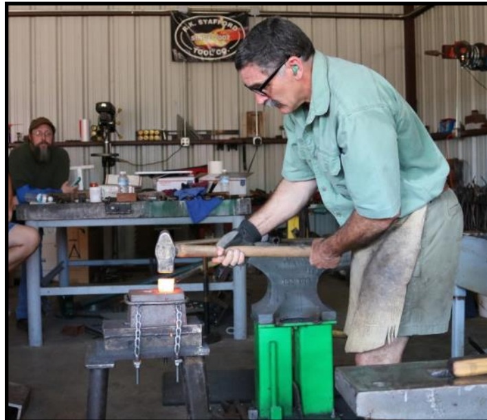
Mark forging a bottom tool blank in an upsetting block
