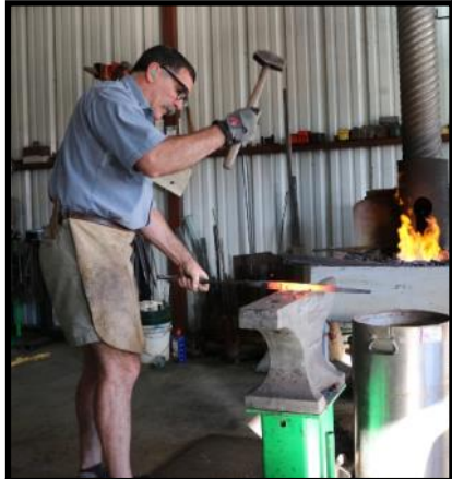
Mark forging the large hammer eye drift from a Klein Bullpin
