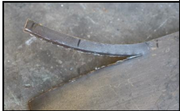
Cold cut about 4" long in a scrap piece of 1/8" sheet steel to demonstrate the toughness of the newly forged slitting chisel.
