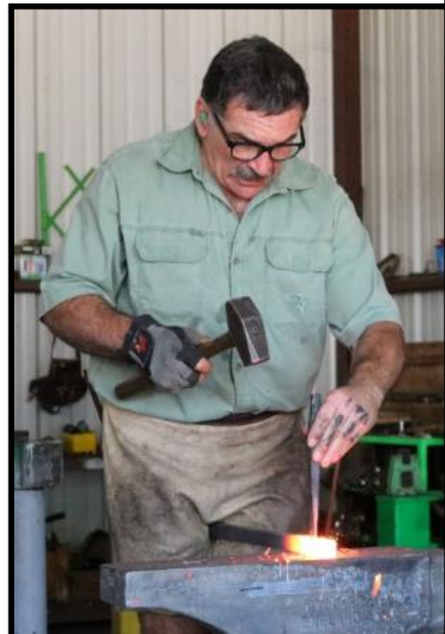
Mark slot punching the leafing hammer eye
