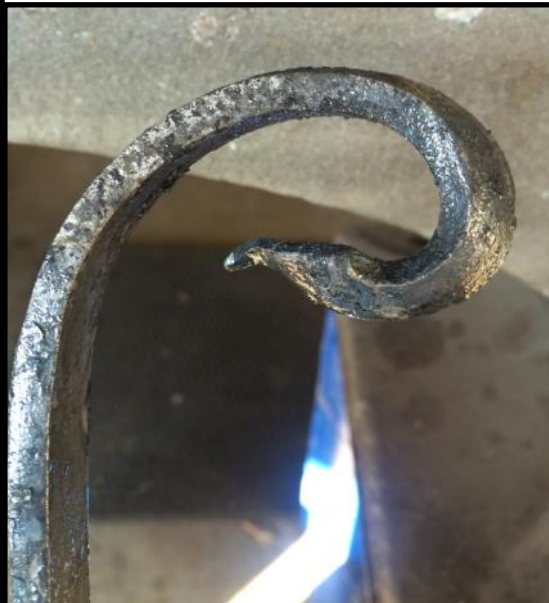
The blown over beveled leaf scroll from the ABANA National Curriculum Grille Project
