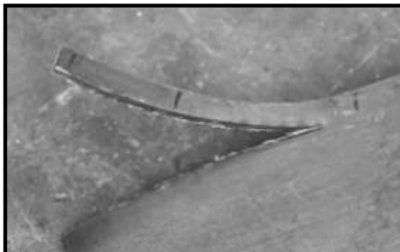
Cold cut about 4" long in a scrap piece of 1/8" sheet steel to demonstrate the toughness of the newly forged slitting chisel.
