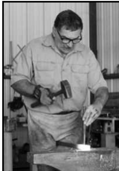
Mark slot punching the leafing hammer eye
