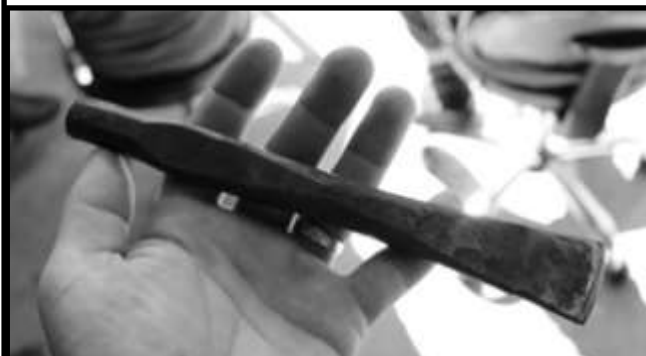
Mark Aspery style hot slitting chisel forged and heat treated at the Brookhaven demo
