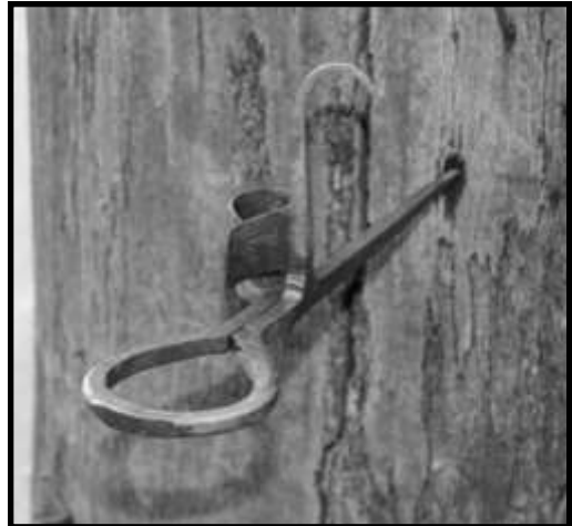
The finished candlestick tapped into the anvil block. Notice the upset corners where the bend comes together.
