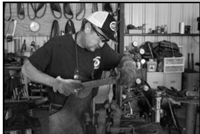
Mark Carter hot rasping the leafing hammer face
