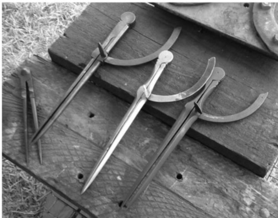
FIG. 2. TWO EXAMPLES OF COMPASS LEAVES. THE ONE ON THE LEFT WOULD BE SLIT AS IN THE ONE THAT PETER WAS DEMOING AND THE LONGER LEAF ON THE RIGHT WOULD BE BETTER SUITED FOLDED AND WELDED AS HE SHOWS US IN THE DVD.
