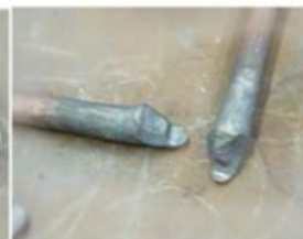
Round to Round scarf weld
