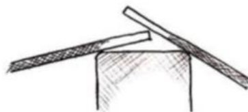
Figure 3: Positioning bars for welding
