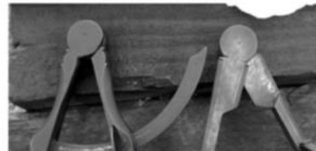
FIG. 2. TWO EXAMPLES OF COMPASS LEAVES. THE ONE ON THE LEFT WOULD BE SLIT AS IN THE ONE THAT PETER WAS DEMOING AND THE LONGER LEAF ON THE RIGHT WOULD BE BETTER SUITED FOLDED AND WELDED AS HE SHOWS US IN THE DVD.
