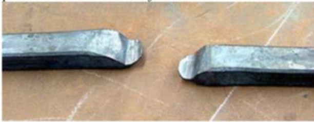
Figure 5: Two scarfed bars ready for welding
