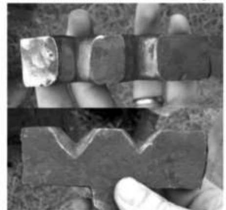
FIG. 3 SHOWS THE TOP AND SIDE VIEWS OF THE V SWAGE THAT PETER USES TO SHAPE THE SHOULDERS AT THE TOP OF THE COMPASS LEG, BOTH BELOW THE HINGE AND ABOVE AND BELOW THE MORTISE FOR THE WING.
