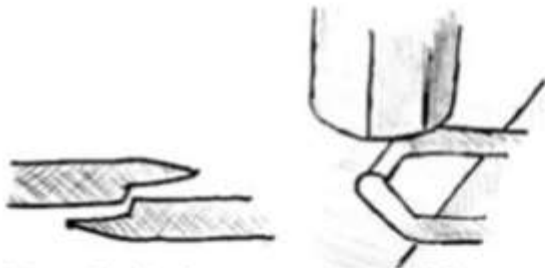
Figure 11: Final position before welding
