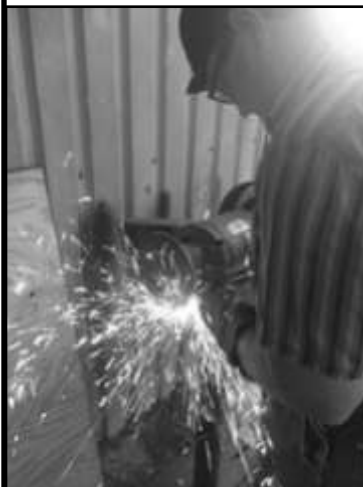
Mandell grinding the outer contour on an eye punch.
