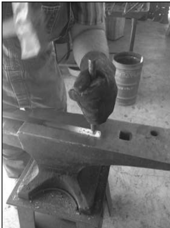
Using the double eye punch on a piece of test stock
