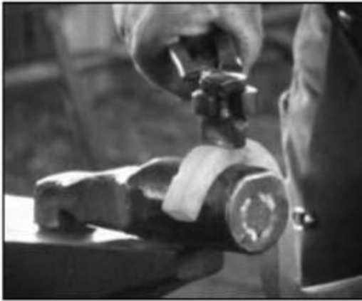
Flatten the base of the mortise. The flatter is smaller than the finished notch floor, move around to get the totally flat floor desired, angling the flatter to follow the layout and cuts.
