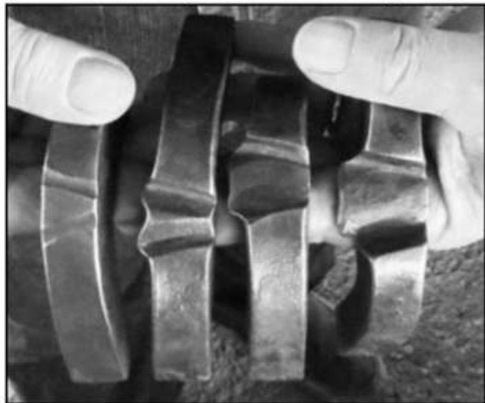
Sometimes it is difficult to do the mortise first, it can be best to leave mass at the base of the mortise and do that part last. Sample pieces showing the progression of mortise forming steps.
