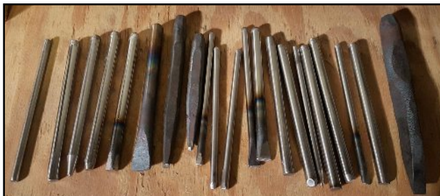
Fig. 7: New Chasing Tools Quickly Made with the Induction Heater
