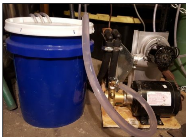
Fig. 4: The Shop Built Water Cooler
