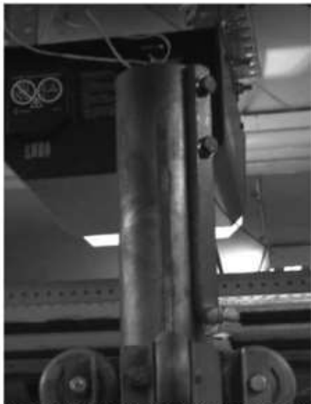
FIG. 4 - MIKE ATTACHED AN 'L' SHAPED STOP TO THE TOP OF HIS TREADLE HAMMER THAT STOPS IT FROM COMING DOWN AND CRUSHING HIS HAND.
