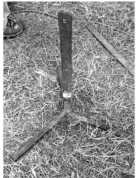
FIG. 6 - THE FINISHED LOWER PORTION OF THE LEG.
