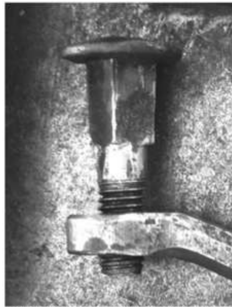
FIG. 3 - CLOSE UP OF THE FINISHED CARRIAGE BOLT.
