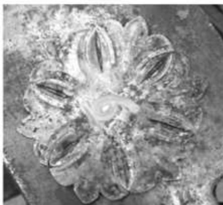
FIG. 6 - MIKE CHISELED A DETAIL DOWN THE PEDALS TO ENHANCE THE DESIGN.
