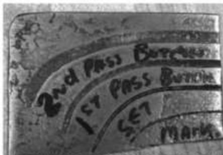
FIG. 7 - MIKE MADE A SAMPLE PIECES SHOWING THE MARKS LEFT BY EACH OF THE TOOLS.
