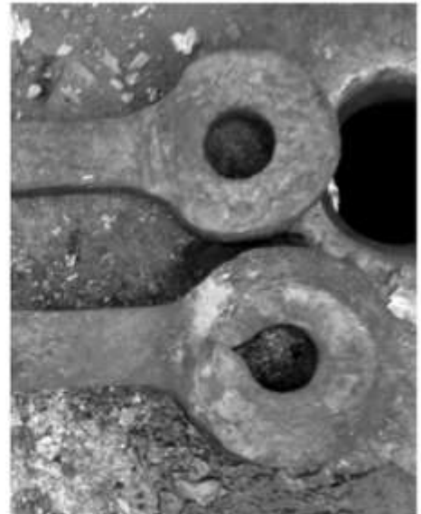
FIG. 5 SHOWS THE TWO METHODS OF SHAPING THE NUT. ALTERNATIVE METHOD ON THE BOTTOM.
