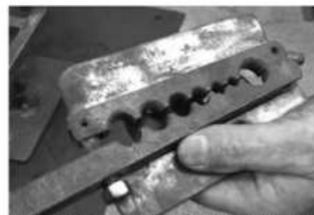
FIG. 9 - THE UNDERSIDE OF MIKE'S HEADING TOOL. AN OLD PIPE FITTING TOOL WITH FLANGES WELDED TO THE TOP
