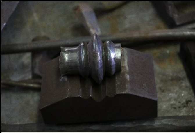
Shape made by rotating the piece in a profile swage.
