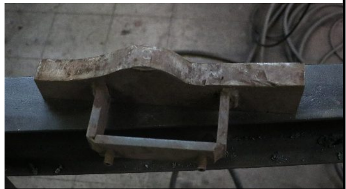
This profiling tool and its mate are designed to be mounted on the front of the dies rather than the face. This allows more space between the tooling than would otherwise be available.
