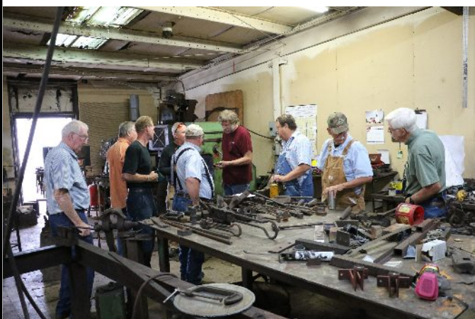
Rick showing some shop made power hammer tooling.
