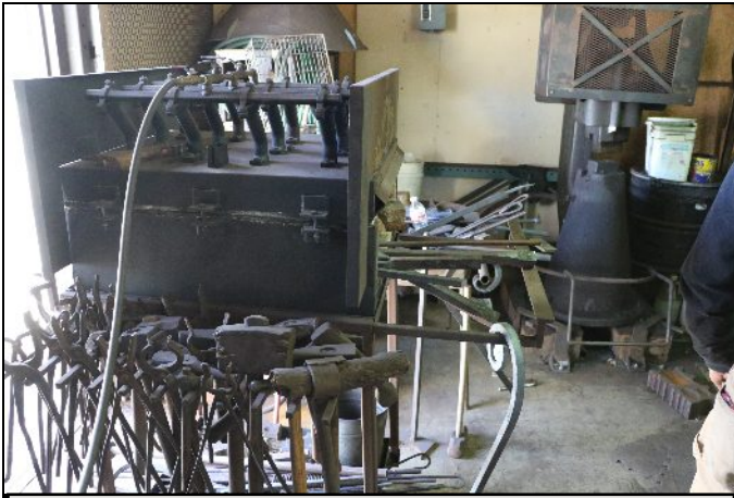
Rick's multi-burner propane production forge.
