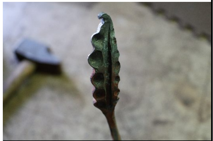
A leaf element textured with the ball pein hammer.
