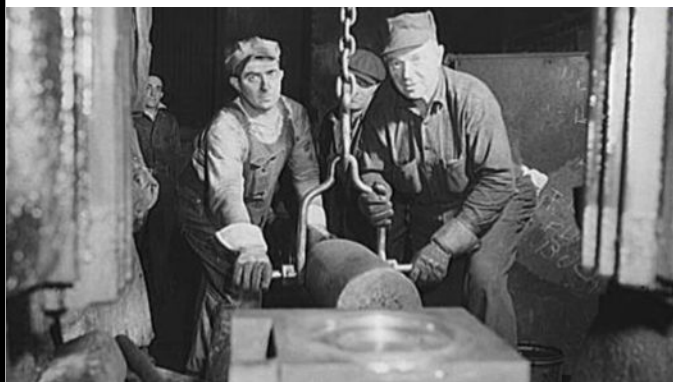
Workers drive a die key on a forging hammer producing heavy hydraulic fittings, to produce boilers for a U.S. military contract.
