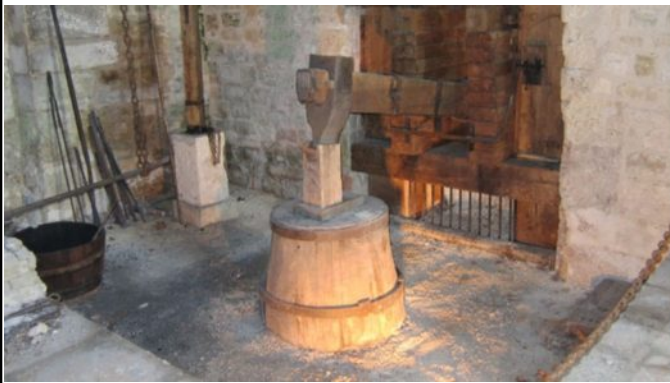
A water-powered hammer in the forge at Fontenay Abbey, near Montbard, France. There, Cistercian monks devised this forging system as early as 1220, to produce iron tools.
