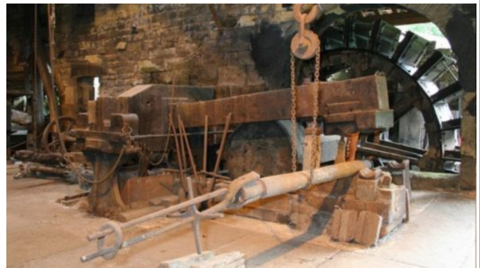
At Wortley Top Forge, near Sheffield, England, this “belly helve hammer” was a 16th-Century water-powered system used to form iron into forgeable bars.
