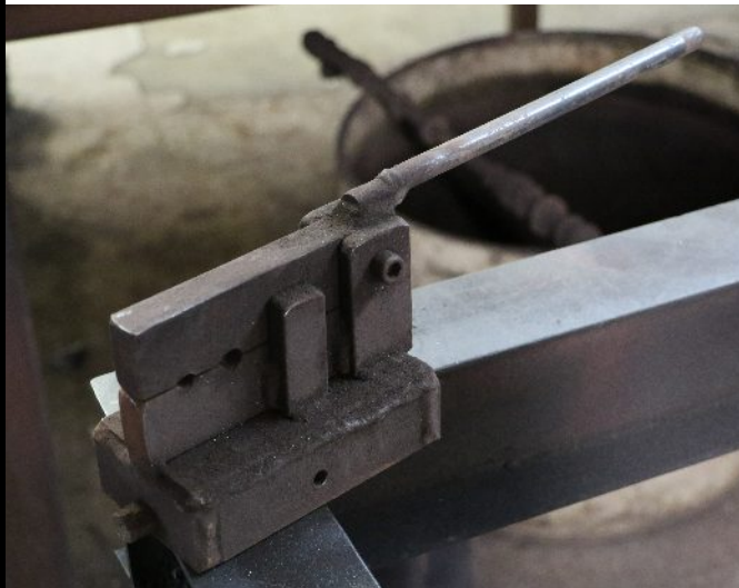
Tenon swage tool with a die mount base and a quick opening handle.
