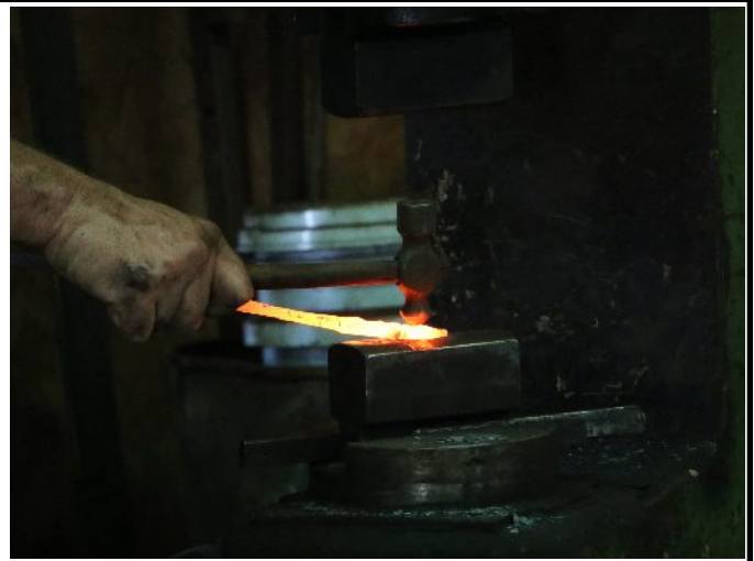
Some power hammer tools can be made from simple tools already available. You might recognize this one as a ball pein hammer.
